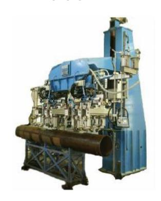
The L-Saw UT test systems is to test the Weld defects based on the International Standard in general API, Shell, Etc.The Test Mechnism will have probe carriege shall be in number 2 to 4 based on the test configration Mode like nos of I-mode, X-mode, Tendom, HAZ, Onbead, etc.
